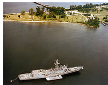
EMPRESS I (antennas along shoreline) with USS Estocin (FFG-15) moored in the foreground for testing.
