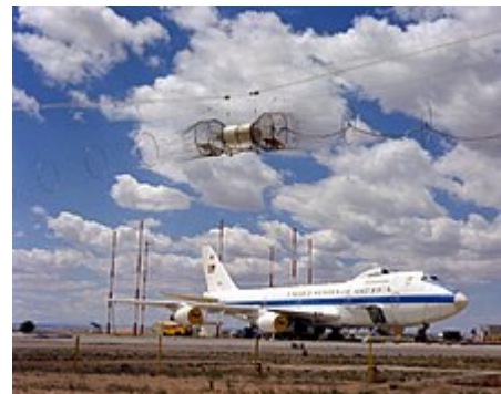
EMP simulator HAGII-C testing a Boeing E-4 aircraft.
