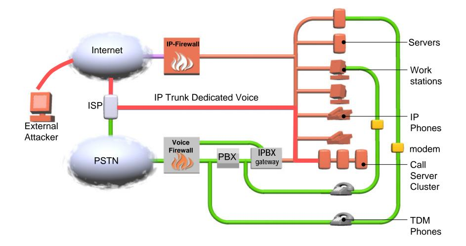
External attack through IP Trunks against IP Voice and Data Network
