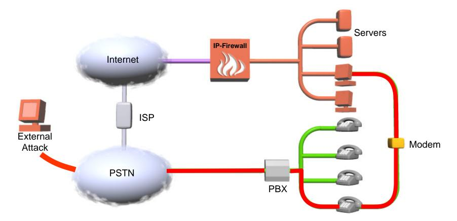
Whitehat Wardialing – 2%-4% of phone lines have unauthorized modems. However, only 20% of UNAUTHORIZED modems detected via Whitehat Wardialing.
